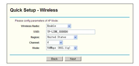
Figure 3-9 Quick Setup - Wireless settings
