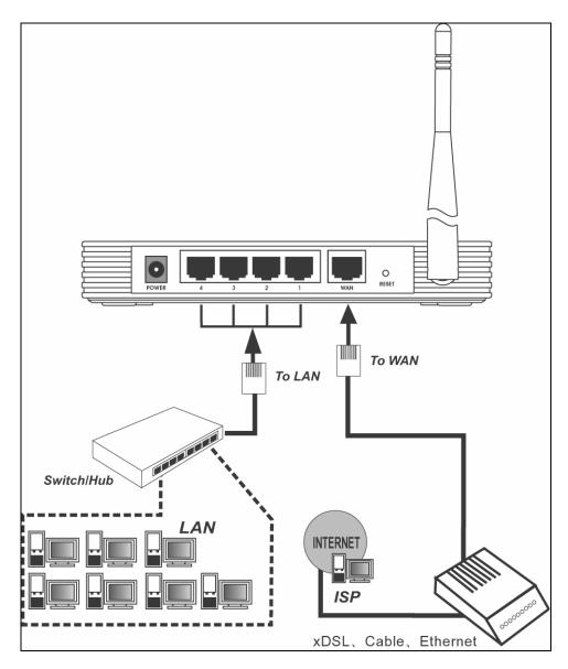
Figure 2-1 Hardware Installation of the TL-WR542G 54Mbps Wireless Router
