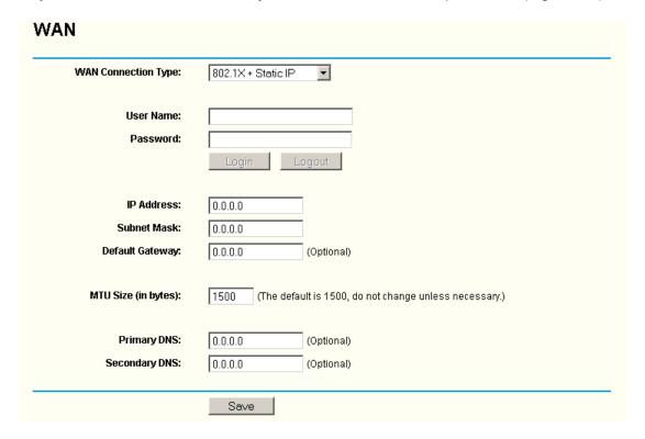
Figure 4-9 802.1X + Static IP Settings
